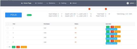
After log-in, the top pane of the page provides the following options for PDU operations: **Home Page**, **Control**, **Statistics**, **Settings**, and **About**. Click the corresponding TAB to select, set, and view the functions provided on the corresponding page.
