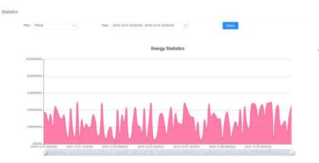
You can collect energy consumption statistics based on the specified query time range. Select a start time from the drop-down list box based on the date, month, and year. You can select energy consumption within 24 hours, the latest 7 days, 30 days, and 90 days based on the quick selection function on the time bar.
