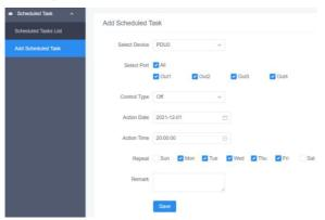
In the add scheduled task TAB, you can add scheduled tasks based on your requirements, such as socket port, switch type, time, working day, and remarks. Select the corresponding option and click the Save button to Save and generate a scheduled task. PDU will perform the corresponding scheduled task operation at the set time.
