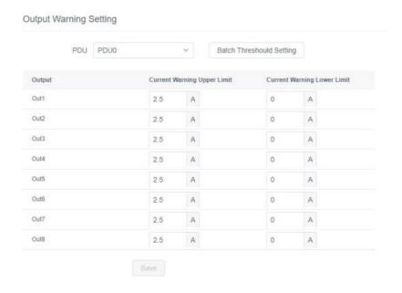
Output Warning setting. You can set the upper limit and lower limit of the output current of each power output port respectively to ensure that the electrical device works within a safe current range. If the output current exceeds the set range, the system will issue an alarm. You can also set parameters in batches. Treat the same setup requirements uniformly.
